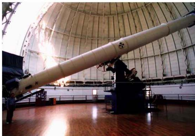
Figure 2.9.6: In 1897, the Yerkes Observatory in Wisconsin (USA) built a large refracting telescope with an objective lens that is 40 inches in diameter and has a tube length of 62 feet. (credit: Yerkes Observatory, University of Chicago)
