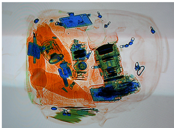
Figure 8.6.9: An X-ray image of a piece of luggage. The denser the material, the darker the shadow. Object colors relate to material composition—metallic objects show up as blue in this image. (credit: "IDuke"/Wikimedia Commons)
