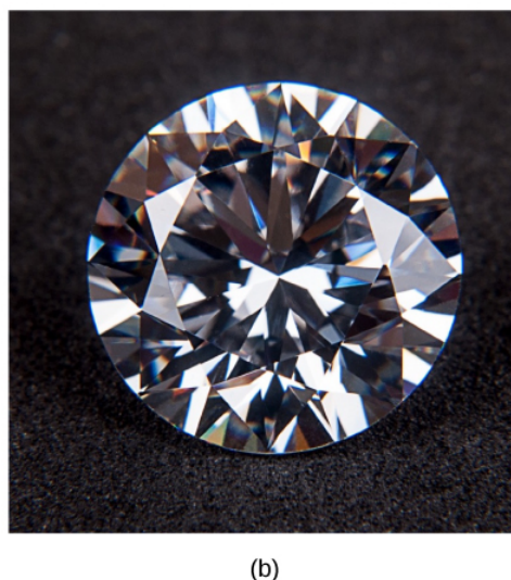
Figure 9.4.5: Structure of the diamond crystal. (a) The single carbon atom represented by the dark blue sphere is covalently bonded to the four carbon atoms represented by the light blue spheres. (b) Gem-quality diamonds can be cleaved along smooth planes, which gives a large number of angles that cause total internal reflection of incident light, and thus gives diamonds their prized brilliance.
