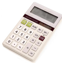
Figure 9.E. 7: The strip of solar cells just above the keys of this calculator convert light to electricity to supply its energy needs. (credit: Evan-Amos, Wikimedia Commons)
