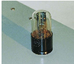
Figure 12.3.2: A photo of a photoelectric effect experiment vacuum tube is shown above. (Credit: P.P. Urone)
