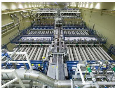
Figure 14.9.9: National Ignition Facility (CA). This image shows a laser bay where 192 laser beams will focus onto a small D-T target, producing fusion. (credit: Lawrence Livermore National Laboratory, Lawrence Livermore National Security, LLC, and the Department of Energy)
