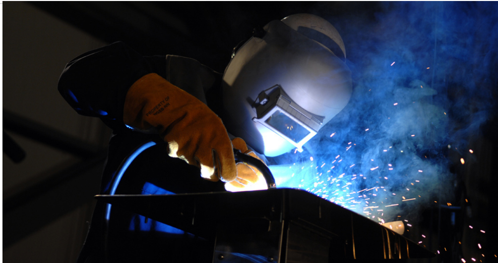
Figure 8.1.1: The welder's gloves and helmet protect him from the electric arc that transfers enough thermal energy to melt the rod, spray sparks, and burn the retina of an unprotected eye. The thermal energy can be felt on exposed skin a few meters away, and its light can be seen for kilometers. (credit: Kevin S. O'Brien/U.S. Navy)
