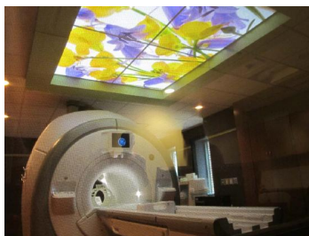
Figure 10.3.3: Instrument for magnetic resonance imaging (MRI). The device uses a superconducting cylindrical coil for the main magnetic field. The patient goes into this “tunnel” on the gurney. (credit: Bill McChesney, Flickr)
