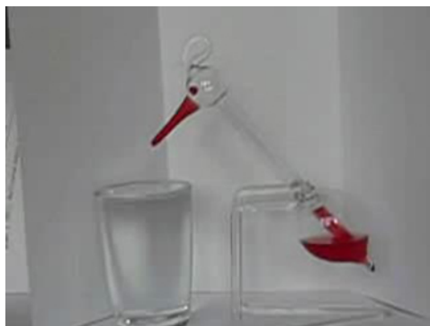
Figure 8.11.1: This novelty toy, known as the drinking bird, is an example of Carnot's engine. It contains methylene chloride (mixed with a dye) in the abdomen, which boils at a very low temperature—about 100°F. To operate, one gets the bird's head wet. As the water evaporates, fluid moves up into the head, causing the bird to become top-heavy and dip forward back into the water. This cools down the methylene chloride in the head, and it moves back into the abdomen, causing the bird to become bottom heavy and tip up. Except for a very small input of energy—the original head-wetting—the bird becomes a perpetual motion machine of sorts. (credit: Arabesk.nl, Wikimedia Commons)
