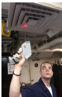
Figure 8.2.3: Fireman Jason Ormand uses a pyrometer to check the temperature of an aircraft carrier's ventilation system. Infrared radiation (whose emission varies with temperature) from the vent is measured and a temperature readout is quickly produced. Infrared measurements are also frequently used as a measure of body temperature. These modern thermometers, placed in the ear canal, are more accurate than alcohol thermometers placed under the tongue or in the armpit. (credit: Lamel J. Hinton/U.S. Navy)
