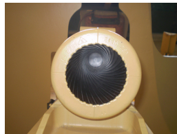
Figure 6.E. 5: The image shows a view down the barrel of a cannon, emphasizing its rifling. Rifling in the barrel of a canon causes the projectile to spin just as is the case for rifles (hence the name for the grooves in the barrel). (credit: Elsie esq., Flickr)
