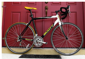
Figure 6.E. 1: The image shows a side view of a racing bicycle. Can you see evidence in the design of the wheels on this racing bicycle that their moment of inertia has been purposely reduced? (credit: Jesús Rodríguez)
