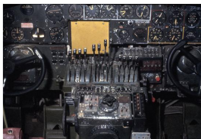
Figure 14.2.1: The dials of this World War II aircraft will glow in the dark, because they are painted with radium-doped phosphorescent paint. It is a poignant reminder of the dual nature of radiation. Although radium paint dials are conveniently visible day and night, they emit radon, a hazardous radioactive gas that is odorless, colorless, and tasteless. (credit: U.S. Air Force Photo)
