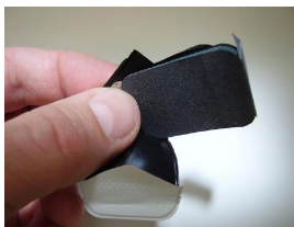
Figure 14.3.1: Film badges contain film similar to that used in this dental x-ray film and is sandwiched between various absorbers to determine the penetrating ability of the radiation as well as the amount. (credit: Werneuchen, Wikimedia Commons)
