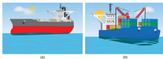
Figure 7.6.4: An unloaded ship (a) floats higher in the water than a loaded ship (b).
