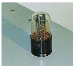
Figure 12.3.2: A photo of a photoelectric effect experiment vacuum tube is shown above. (Credit: P.P. Urone)
