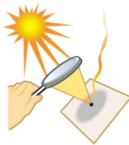
Figure 11.9.2: Sunlight focused by a converging magnifying glass can burn paper. Light rays from the sun are nearly parallel and cross at the focal point of the lens. The more powerful the lens, the closer to the lens the rays will cross.
