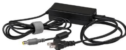
Figure 7.3.1: This power adapter uses metal wires and connectors to conduct electricity from the wall socket to a laptop computer. The conducting wires allow electrons to move freely through the cables, which are shielded by rubber and plastic. These materials act as insulators that don't allow electric charge to escape outward. (credit: Evan-Amos, Wikimedia Commons)
