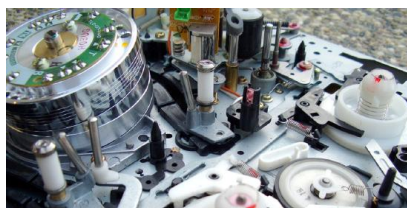
Figure 10.3.2: Recording and playback heads used with audio and video magnetic tapes. (credit: Steve Jurvetson)
