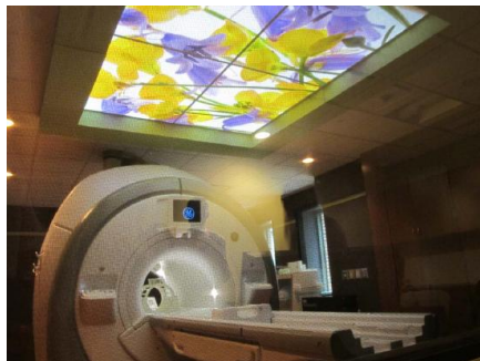
Figure 9.3.3: Instrument for magnetic resonance imaging (MRI). The device uses a superconducting cylindrical coil for the main magnetic field. The patient goes into this “tunnel” on the gurney. (credit: Bill McChesney, Flickr)
