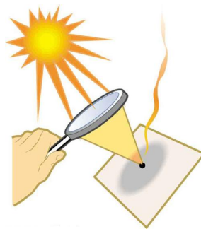
Figure 11.6.2: Sunlight focused by a converging magnifying glass can burn paper. Light rays from the sun are nearly parallel and cross at the focal point of the lens. The more powerful the lens, the closer to the lens the rays will cross.
