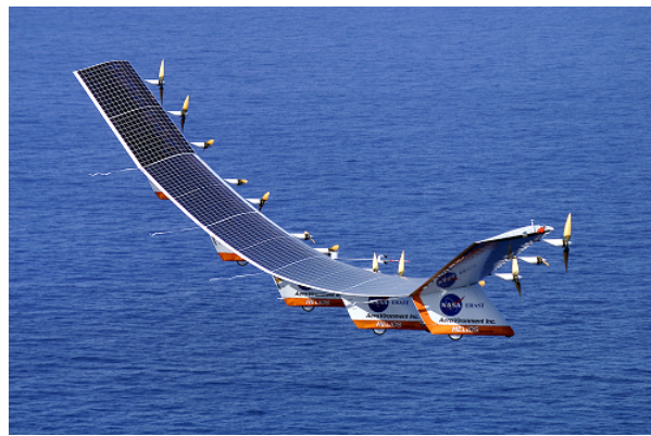
Figure 3.5.1: Solar energy is converted into electrical energy by solar cells, which is used to run a motor in this solar-power aircraft. (credit: NASA)
