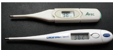
Figure 8.4.3: These familiar thermometers are based on the automated measurement of a thermistor's temperature-dependent resistance. (credit: Biol, Wikimedia Commons)
