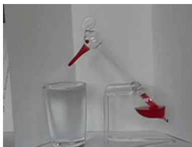
Figure 12.5.1: This novelty toy, known as the drinking bird, is an example of Carnot's engine. It contains methylene chloride (mixed with a dye) in the abdomen, which boils at a very low temperature—about 100^\circ F . To operate, one gets the bird's head wet. As the water evaporates, fluid moves up into the head, causing the bird to become top-heavy and dip forward back into the water. This cools down the methylene chloride in the head, and it moves back into the abdomen, causing the bird to become bottom heavy and tip up. Except for a very small input of energy—the original head-wetting—the bird becomes a perpetual motion machine of sorts. (credit: Arabesk.nl, Wikimedia Commons)
