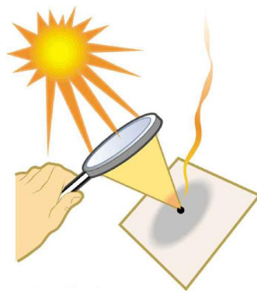
Figure 11.6.2: Sunlight focused by a converging magnifying glass can burn paper. Light rays from the sun are nearly parallel and cross at the focal point of the lens. The more powerful the lens, the closer to the lens the rays will cross.
