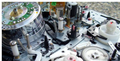
Figure 10.3.2: Recording and playback heads used with audio and video magnetic tapes. (credit: Steve Jurvetson)
