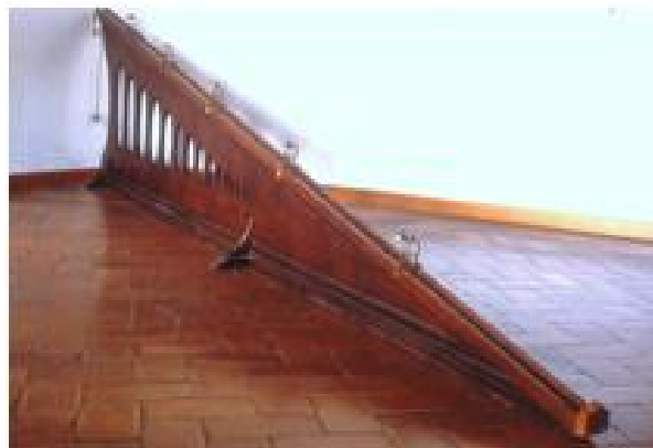
Figure 7.1: Galileo's Experimental Apparatus. Galileo used experiments based upon systems similar to this one to study the motion of falling objects. He also studied the motions of pendula, finding that their periods depend only upon their length, not upon the mass of the object suspended. Credit: Museo Galileo, Florence - Photo Franca Principe
