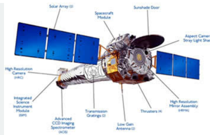
Figure B.3 The parts of the Chandra Observatory. To see an interactive version of this figure, click here . Mouse over the different parts to learn more details. Credit: NASA/CXC.
