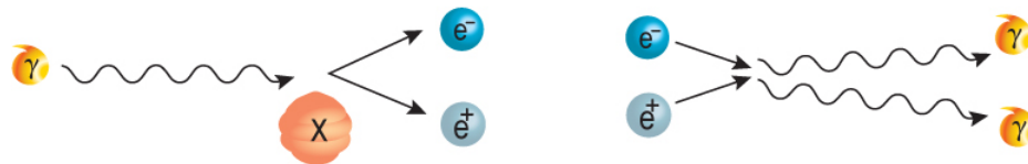
Figure 16.15: At high enough energies it is possible for a photon to spontaneously convert its energy into particles. The process must involve another particle, which must carry away some of the momentum of the photon. The opposite process, annihilation, occurs when a positron and electron combine to form a pair of photons. Each photon carries the energy of the rest mass of one of the original particles, thus conserving energy. However, two photons must be created in order to conserve the momentum of the original particles. Credit: NASA/SSU/Aurore Simonnet
