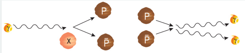
Figure A.16.2: At high temperatures photons spontaneously produce a proton and an antiproton, as shown at left. The particles will quickly combine with other protons or antiprotons and annihilate, as shown at right, creating two photons. These two processes keep each other in balance until the temperature drops to the point that photons are no longer energetic enough to produce the proton—antiproton pairs. Credit: NASA/SSU/Aurore Simonnet
