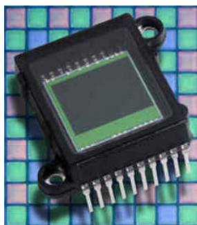
Figure 3.1: This image shows a charge-coupled device, or CCD chip. The dark rectangle at the center of the chip is the array of pixels that detect individual photons. The pins read out the electrical charge produced by the light to a digital camera, and electronic circuitry inside the camera converts the charge into an image that can be viewed on a computer screen. Credit: NASA.
