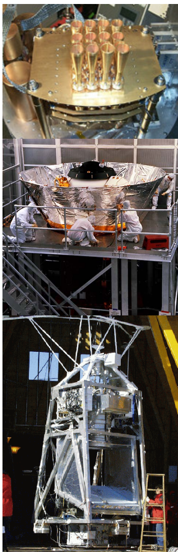
Figure 15.9a: A few of the many instruments used in recent CMB experiments: a close-up of the ACBAR feed horns and electronics, the BOOMERANG telescope , and the WMAP satellite. To date there have been more than 50 experiments designed to measure the CMB. Credits: Acbar Collaboration, NASA/COBE Team, BOOMERANG Collaboration
