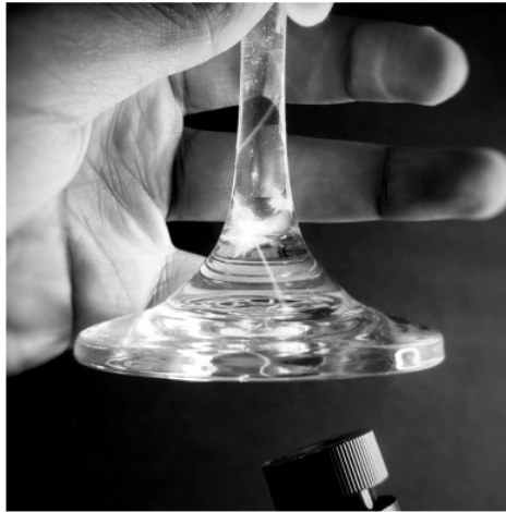
Figure 1.11.2: Light guided within a piece of glass. (from Wikimedia Commons by Keerthi - CC BY ).
