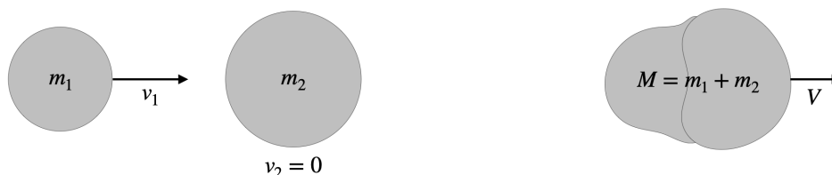
Figure 4.4.1 – Perfectly Inelastic Collision
