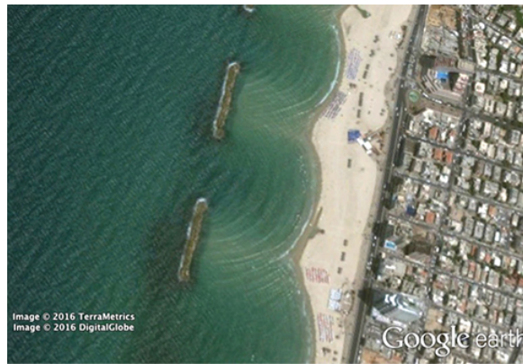
Figure 4.2.1: Because of the diffraction of waves, ocean waves entering through an opening in a breakwater can spread throughout the bay. (credit: modification of map data from Google Earth)
