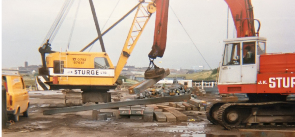
Figure 6.1.1: An industrial electromagnet is capable of lifting thousands of pounds of metallic waste. (credit: modification of work by "BedfordAI"/Flickr)
