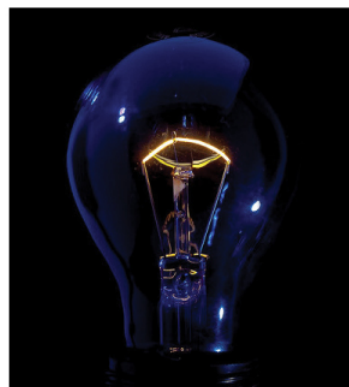
Figure 4.3.3: The incandescent lamp is a simple design. A tungsten filament is placed in a partially evacuated glass envelope. One end of the filament is attached to the screw base, which is made out of a conducting material. The second end of the filament is attached to a second contact in the base of the bulb. The two contacts are separated by an insulating material. Current flows through the filament, and the temperature of the filament becomes large enough to cause the filament to glow and produce light. However, these bulbs are not very energy efficient, as evident from the heat coming from the bulb. In the year 2012, the United States, along with many other countries, began to phase out incandescent lamps in favor of more energy-efficient lamps, such as light-emitting diode (LED) lamps and compact fluorescent lamps (CFL) (credit right: modification of work by Serge Saint).
