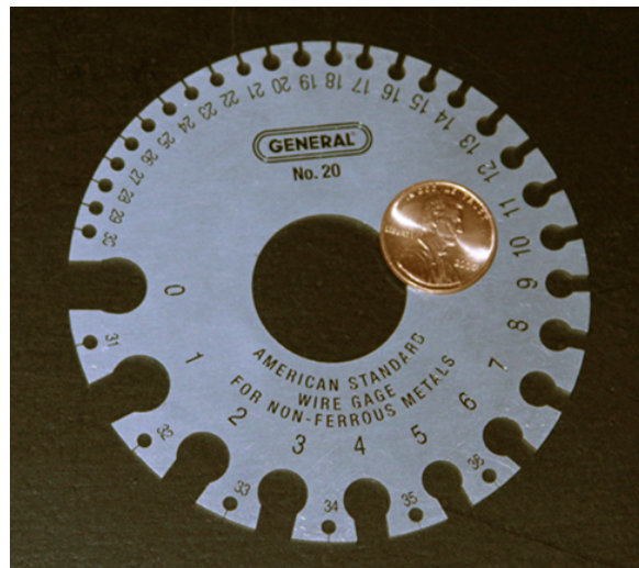
Figure 4.3.5: A device for measuring the gauge of electrical wire. As you can see, higher gauge numbers indicate thinner wires.
