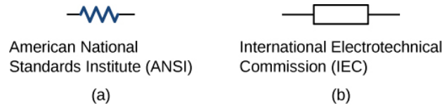
Figure 4.4.2: Symbols for a resistor used in circuit diagrams. (a) The ANSI symbol; (b) the IEC symbol.
