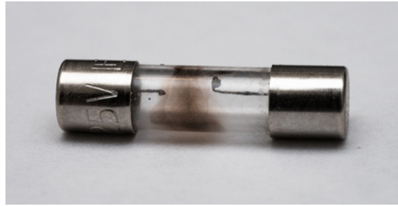
Figure 4.6.3: A fuse consists of a piece of wire between two contacts. When a current passes through the wire that is greater than the rated current, the wire melts, breaking the connection. Pictured is a “blown” fuse where the wire broke protecting a circuit (credit: modification of work by “Shardayy”/Flickr).
