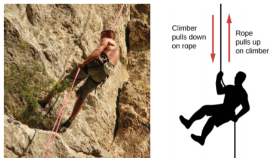
Figure 14.4.2: When the mountain climber pulls down on the rope, the rope pulls up on the mountain climber.
