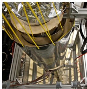
Figure 1.3.2: An atomic clock such as this one uses the vibrations of cesium atoms to keep time to a precision of better than a microsecond per year. The fundamental unit of time, the second, is based on such clocks. This image looks down from the top of an atomic fountain nearly 30 feet tall. (credit: Steve Jurvetson)
