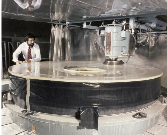
Grinding of the Hubble Space Telescope Mirror, 1979Public Domain | Image courtesy of NASA.
