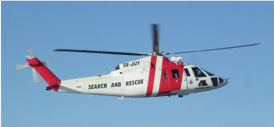
Figure 10.7.1: A helicopter has its main lift blades rotating to keep the aircraft airborne. Due to conservation of angular momentum, the body of the helicopter would want to rotate in the opposite sense to the blades, if it were not for the small rotor on the tail of the aircraft, which provides thrust to stabilize it.
