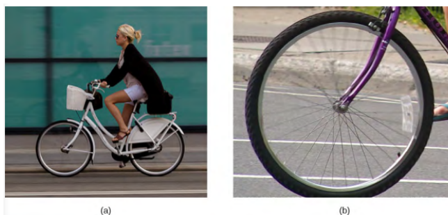
Figure 9.16.1: (a) The bicycle moves forward, and its tires do not slip. The bottom of the slightly deformed tire is at rest with respect to the road surface for a measurable amount of time. (b) This image shows that the top of a rolling wheel appears blurred by its motion, but the bottom of the wheel is instantaneously at rest. (credit a: modification of work by Nelson Lourenço; credit b: modification of work by Colin Rose)
