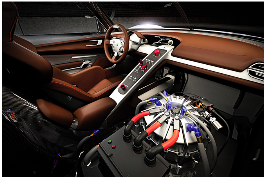
Figure 9.3.2: A KERS (kinetic energy recovery system) flywheel used in cars. (credit: “cmonville”/Flickr)
