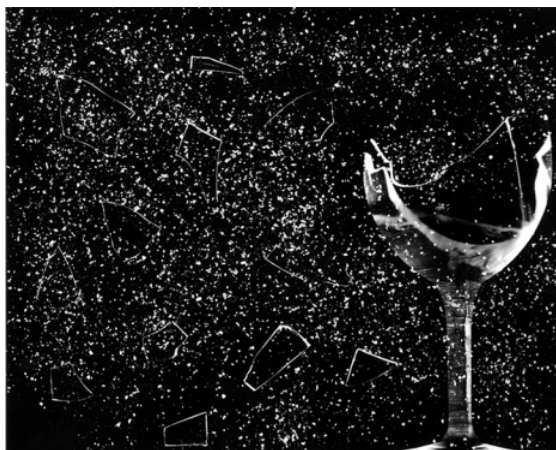
Figure 12.5.1: This glass has been shattered by a high-intensity sound wave of the same frequency as the resonant frequency of the glass. (credit: "||read||"/Flickr)
