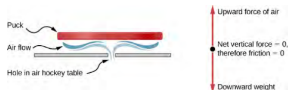
Figure 6.1.2: An air hockey table is useful in illustrating Newton's laws. When the air is off, friction quickly slows the puck; but when the air is on, it minimizes contact between the puck and the hockey table, and the puck glides far down the table.
