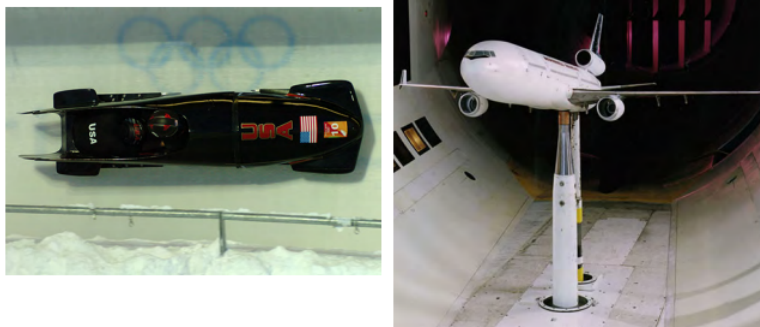
Figure 6.6.1: (A) From racing cars to bobsled racers, aerodynamic shaping is crucial to achieving top speeds. Bobsleds are designed for speed and are shaped like a bullet with tapered fins. (credit: "U.S. Army"/Wikimedia Commons) (B): NASA researchers test a model plane in a wind tunnel. (credit: NASA/Ames).
