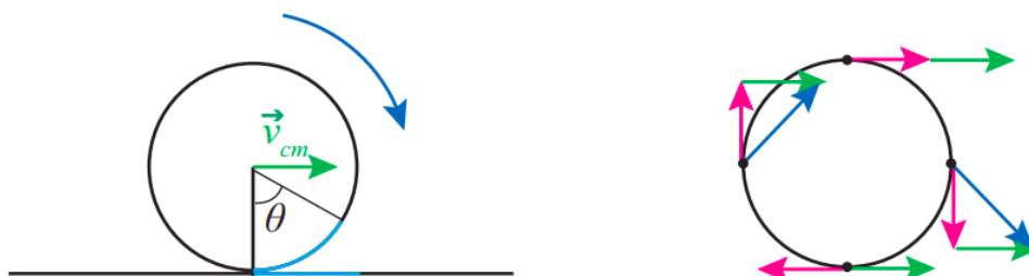
Figure 9.4.1: Left: illustrating the rolling without slipping condition. The cyan line on the surface has the same length as the cyan-colored arc, and will be the distance traveled by the disk when it has turned through an angle \theta . Right: velocities for four points on the edge of the disk. The pink arrows are the velocities in the center of mass frame. In the Earth reference frame, the velocity of the center of mass, \vec{v}_{cm} , in green, has to be added to each of them. The resultant is shown in blue for two of them.
