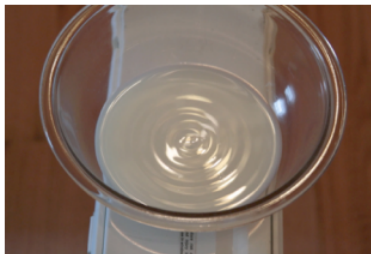
Figure 12.8.1: Standing waves are formed on the surface of a bowl of milk sitting on a box fan. The vibrations from the fan causes the surface of the milk to oscillate. The waves are visible due to the reflection of light from a lamp.
