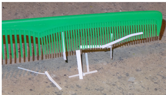
Figure 3.1.2: After being used to comb hair, this comb attracts small strips of paper from a distance, without physical contact. Investigation of this behavior helped lead to the concept of the electric force.
