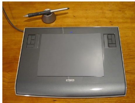
Figure 8.7.1: A tablet with a specially designed pen to write with is another application of magnetic induction.
