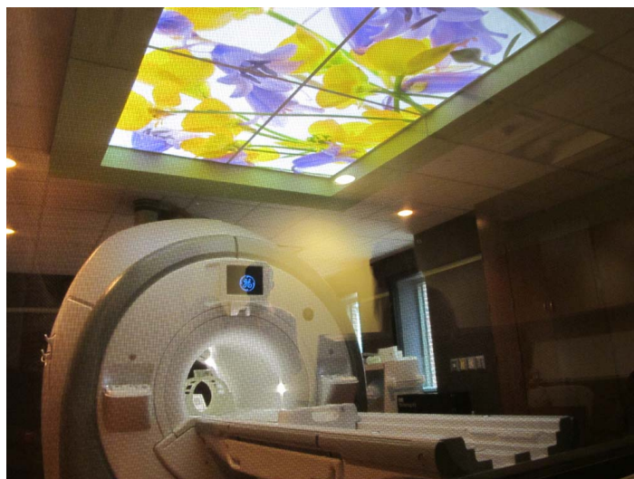
Figure 7.2.3: Instrument for magnetic resonance imaging (MRI). The device uses a superconducting cylindrical coil for the main magnetic field. The patient goes into this “tunnel” on the gurney. (credit: Bill McChesney, Flickr)
