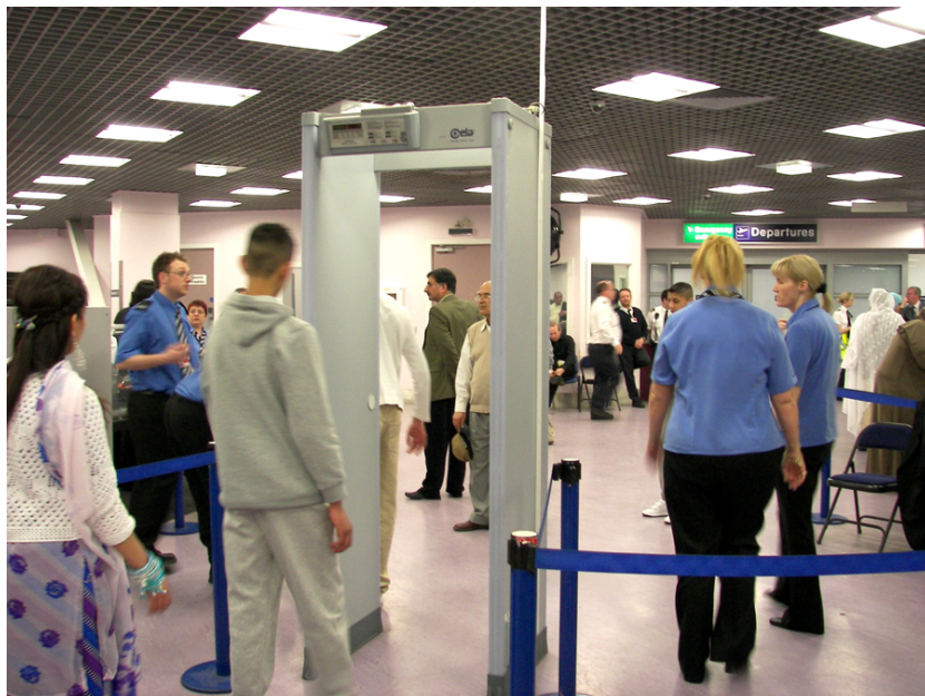
Figure 8.6.5: The familiar security gate at an airport can not only detect metals but also indicate their approximate height above the floor. (credit: Alexbuidrds, Wikimedia Commons)
