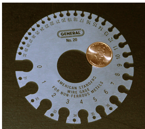
Figure 5.2.5: A device for measuring the gauge of electrical wire. As you can see, higher gauge numbers indicate thinner wires.
