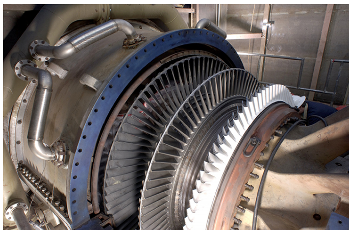
Figure 8.5.5: Steam turbine/generator. The steam produced by burning coal impacts the turbine blades, turning the shaft, which is connected to the generator.
