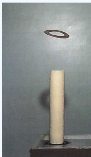
Figure 8.1.9: The jumping ring. When a current is turned on in the vertical solenoid, a current is induced in the metal ring. The stray field produced by the solenoid causes the ring to jump off the solenoid.
