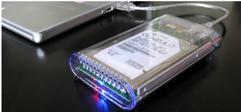
Figure 7.1.1: An external hard drive attached to a computer works by magnetically encoding information that can be stored or retrieved quickly. A key idea in the development of digital devices is the ability to produce and use magnetic fields in this way. (credit: modification of work by “Miss Karen”/Flickr)
