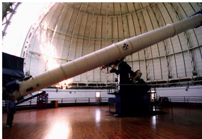
Figure 10.7.6: In 1897, the Yerkes Observatory in Wisconsin (USA) built a large refracting telescope with an objective lens that is 40 inches in diameter and has a tube length of 62 feet. (credit: Yerkes Observatory, University of Chicago)
