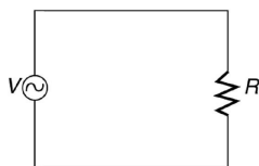
Figure 8.8.1: Schematic of a simple AC circuit with a voltage source and a single appliance represented by the resistance R . There are no safety features in this circuit.
