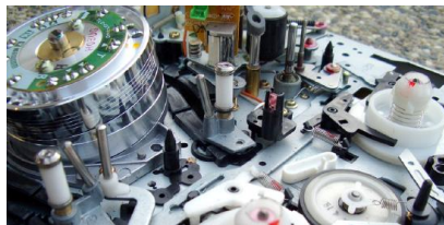
Figure 8.1.2: Recording and playback heads used with audio and video magnetic tapes. (credit: Steve Jurvetson)
