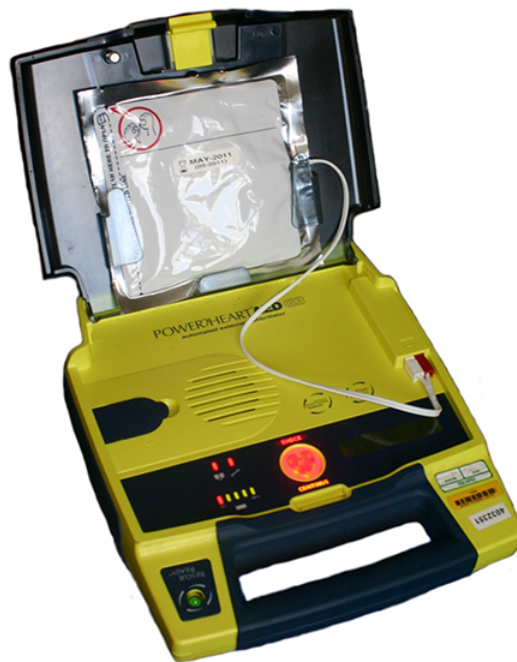
Figure 4.8.2: Automated external defibrillators are found in many public places. These portable units provide verbal instructions for use in the important first few minutes for a person suffering a cardiac attack.
