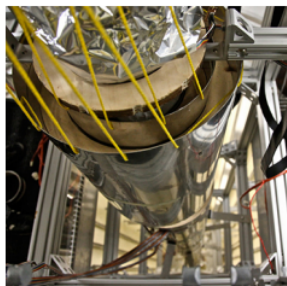
Figure 1.4.2: An atomic clock such as this one uses the vibrations of cesium atoms to keep time to a precision of better than a microsecond per year. The fundamental unit of time, the second, is based on such clocks. This image looks down from the top of an atomic fountain nearly 30 feet tall. (credit: Steve Jurvetson)
