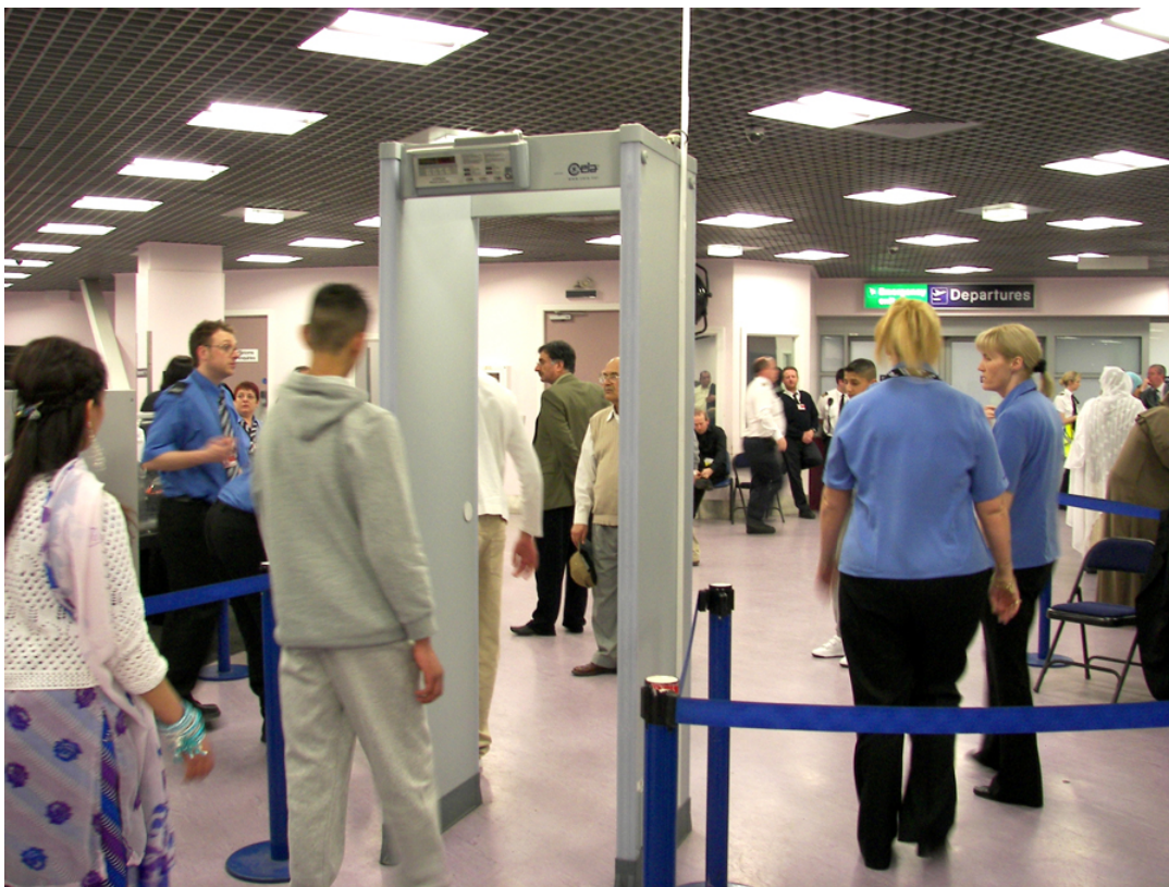
Figure 8.13.5: The familiar security gate at an airport can not only detect metals but also indicate their approximate height above the floor. (credit: Alexbuids, Wikimedia Commons)
