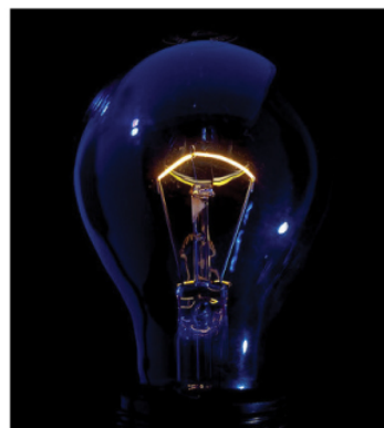
Figure 5.4.3: The incandescent lamp is a simple design. A tungsten filament is placed in a partially evacuated glass envelope. One end of the filament is attached to the screw base, which is made out of a conducting material. The second end of the filament is attached to a second contact in the base of the bulb. The two contacts are separated by an insulating material. Current flows through the filament, and the temperature of the filament becomes large enough to cause the filament to glow and produce light. However, these bulbs are not very energy efficient, as evident from the heat coming from the bulb. In the year 2012, the United States, along with many other countries, began to phase out incandescent lamps in favor of more energy-efficient lamps, such as light-emitting diode (LED) lamps and compact fluorescent lamps (CFL) (credit right: modification of work by Serge Saint).
