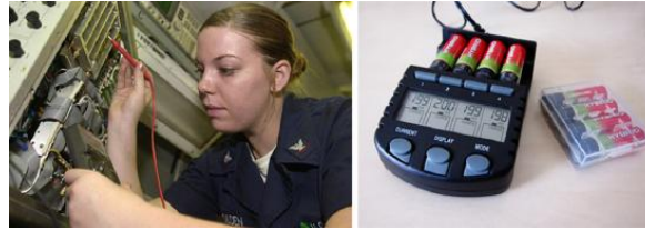
Figure 6.7.3.6: These two battery testers measure terminal voltage under a load to determine the condition of a battery. The large device is being used by a U.S. Navy electronics technician to test large batteries aboard the aircraft carrier USS Nimitz and has a small resistance that can dissipate large amounts of power. (credit: U.S. Navy photo by Photographer's Mate Airman Jason A. Johnston) The small device is used on small batteries and has a digital display to indicate the acceptability of their terminal voltage. (credit: Keith Williamson)
