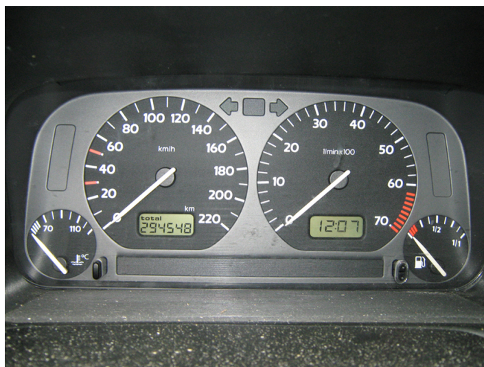
Figure 6.7.5.1: The fuel and temperature gauges (far right and far left, respectively) in this 1996 Volkswagen are voltmeters that register the voltage output of “sender” units, which are hopefully proportional to the amount of gasoline in the tank and the engine temperature. (credit: Christian Giersing)
