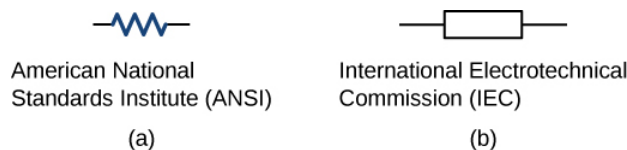
Figure 5.6.2: Symbols for a resistor used in circuit diagrams. (a) The ANSI symbol; (b) the IEC symbol.
