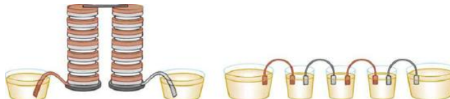
Figure 6.7.3.9: Batteries are multiple connections of individual cells, as shown in this modern rendition of an old print. Single cells, such as AA or C cells, are commonly called batteries, although this is technically incorrect.
