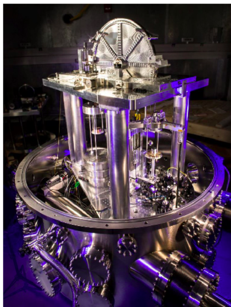
Figure 1.4.4: Redefining the SI unit of mass. The U.S. National Institute of Standards and Technology’s Kibble balance is a machine that balances the weight of a test mass with the resulting electrical current needed for a force to balance it.
