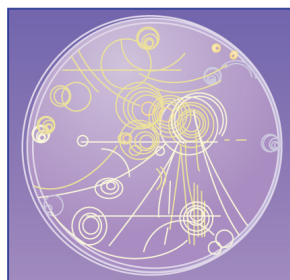
Figure 7.6.1: Trails of bubbles are produced by high-energy charged particles moving through the superheated liquid hydrogen in this artist's rendition of a bubble chamber. There is a strong magnetic field perpendicular to the page that causes the curved paths of the particles. The radius of the path can be used to find the mass, charge, and energy of the particle.
