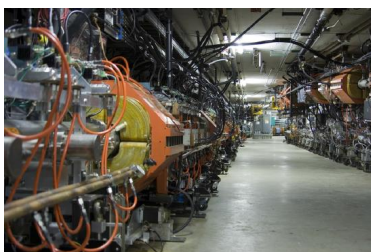
Figure 7.6.7: The Fermilab facility in Illinois has a large particle accelerator (the most powerful in the world until 2008) that employs magnetic fields (magnets seen here in orange) to contain and direct its beam. This and other accelerators have been in use for several decades and have allowed us to discover some of the laws underlying all matter. (credit: ammcgrim, Flickr)
