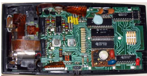
Figure 4.9.1: Energy stored in the large capacitor is used to preserve the memory of an electronic calculator when its batteries are charged. (credit: Kucharek, Wikimedia Commons)
