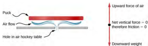
Figure 15.2.2: An air hockey table is useful in illustrating Newton's laws. When the air is off, friction quickly slows the puck; but when the air is on, it minimizes contact between the puck and the hockey table, and the puck glides far down the table.
