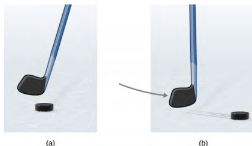
Figure 15.2.1: (a) A hockey puck is shown at rest; it remains at rest until an outside force such as a hockey stick changes its state of rest; (b) a hockey puck is shown in motion; it continues in motion in a straight line until an outside force causes it to change its state of motion. Although it is slick, an ice surface provides some friction that slows the puck.
