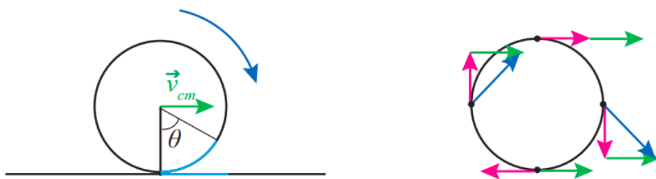
Figure 11.2.1: Left: illustrating the rolling without slipping condition. The cyan line on the surface has the same length as the cyan-colored arc, and will be the distance traveled by the disk when it has turned through an angle \theta . Right: velocities for four points on the edge of the disk. The pink arrows are the velocities in the center of mass frame. In the Earth reference frame, the velocity of the center of mass, \vec{v}_{cm} , in green, has to be added to each of them. The resultant is shown in blue for two of them.
