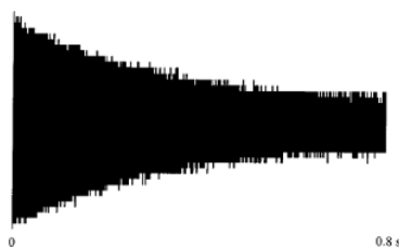
Figure 6.4.6: Signal of a ^{56}\text{Fe}^+ ion in the Orbitrap [6]
