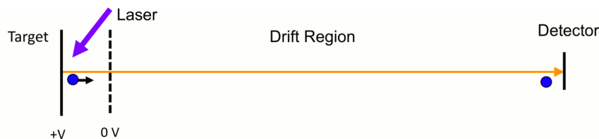
Figure 6.5.2: Schematic diagram of a linear ToF. Laser ionization time-of-flight mass spectrometer where ions are accelerated and separated by mass in a field-free drift region before detection. (CC BY-SA 4.0; κ. κ. Murray via Wikipedia).
