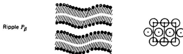
Figure 3.1.4: A depiction of the ripple phase, with a cross-sectional view to the left, and a top view at right illustrating the highly ordered packing arrangement. Note the straight orientation of the fatty acid tails, indicating a low degree of fluidity, similar to the gel phase. (Faller 2015)
