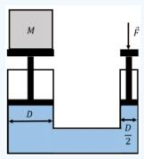
Figure 15.1.8: A force exerted on the piston of a hydraulic lift in order to life a mass M.
