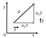
Figure A1.3.2: Illustration that the notation  $\vec{a} = a_x \hat{x} + a_y \hat{y}$  is in fact the vector addition of  $a_x \hat{x}$  and  $a_y \hat{y}$ .
