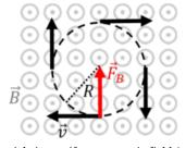
Figure 21.2.2: The motion of a charged particle in a uniform magnetic field (out of the page) is uniform circular motion.
