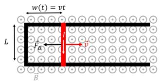
Figure 23.2.1: A U-shaped rail on top of which a bar of length, L, can slide. The system is immersed in a magnetic field that points out of the page. The bar moves to the right with a constant speed v.
