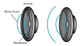
Figure 14.1.6: A speaker creating sound sound waves. The membrane vibrates back and forth which deforms the air to create sound waves that propagate through the air.
