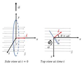
Figure 23.2.2: A loop of wire rotates in a constant and uniform magnetic field. At time t=0 (left panel), the loop lies in the yz plane. The loop rotates about the y axis, with a constant angular velocity,  $\vec{\omega}$ . At some time t later, the loop has rotated through an angle  $\theta=\omega t$  (right panel, as seen from above, looking down on the xz plane).
