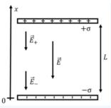
Figure 18.2.2: Two parallel plates with equal and opposite surface charge densities. In the region between the plates, the electric field is uniform.
