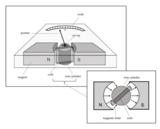
Figure 21.6.3: Illustration of a galvanometer. Current passes through the coil, and the coil rotates due to the torque from a magnetic field created by a permanent magnet. The torque from the magnetic force is balanced by a torsional spring.
