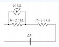
Figure 20.8.2: A circuit with a battery of unknown voltage.
