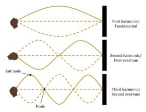
Figure 14.7.1: The first three standing waves on a string.
