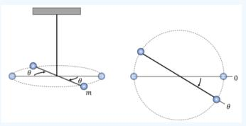
Figure 13.7.4: A torsional pendulum. The right side shows a top view.
