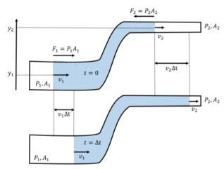
Figure 15.3.4: Laminar flow of an incompressible fluid through a pipe that changes cross-sectional area and height in the direction of flow. An element of fluid, in blue, is shown at time t=0 (top panel), and then, at a later time,  $t=\Delta t$  (bottom panel).
