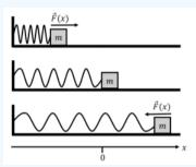
Figure 8.9.3: A mass attached to a spring oscillates about the rest position of the spring.
