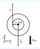
Figure 12.6.2: Free body diagram for the yo-yo.
