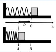
Figure 8.3.2: A block is launched along a frictionless surface by compressing a spring by a distance D. The top panel shows the spring when at rest, and the bottom panel shows the spring compressed by a distance D just before releasing the block.
