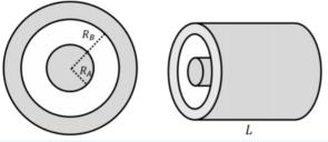
Figure 18.8.1: A capacitor constructed from concentric cylinders.
