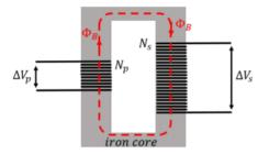
Figure 23.5.1: A transformer converts a primary alternating voltage,  $\Delta V_p$ , to a secondary alternating voltage,  $\Delta V_s$ . The magnetic flux produced in one coil is transmitted by an iron core to the secondary coil, where a different voltage is induced, depending on the ratio of the number of windings in each coil.
