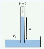
Figure 15.1.12: A Torricelli barometer.
