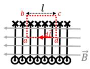
Figure 22.4.3: We use Ampere's Law with a rectangular loop to evaluate the strength of the magnetic field inside a solenoid.
