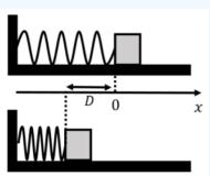
Figure 7.2.2: A block is pressed against a horizontal spring so as to compress the spring by a distance D relative to its rest length.
