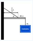
Figure 11.10.2: A sign is suspended on a horizontal bar of mass  ${\cal M}$  and length  ${\cal L}.$
