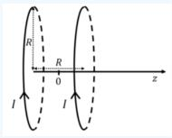
Figure 22.7.2: A Helmholtz coil arrangement.
