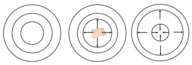
Figure 14.5.3: Left: We divide the air into thin spherical shells. Here we represent three shells (the black circles). Center: When you clap, the innermost shell is given energy and expands. Right: Energy is transferred to the next shell, which expands as the first shell contracts. This is how the wave propagates outwards. When the shells are closer together, the air molecules are closer together and exert a pressure that tries to expand the shell.
