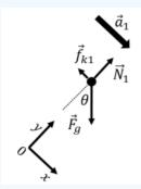
Figure 6.2.3: Free-body diagram for the block when it is on the incline.
