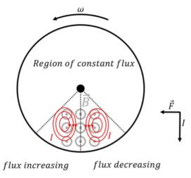
Figure 23.4.3: A rotating wheel made of a conducting material has a small region with a magnetic field. The eddy currents in the region of changing flux result in a net downwards current at the center of the region. The magnetic force that is exerted on that current slows down the wheel.
