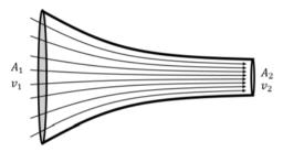
Figure 15.3.2: Laminar flow of a fluid in a narrowing pipe.
