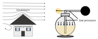
Figure 15.3.6: (Left:) the wind flowing above a roof creates a low pressure zone above the roof. (Right:) air flowing above a vertical spout in the atomizer creates a low pressure zone; the air pressure in the bottle forces the liquid up the spout.
