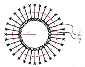
Figure 22.4.5: An Amperian loop of radius r to determine the magnetic field inside of a toroid. Note that the magnetic field everywhere outside the toroid must be zero (think of the current enclosed by Amperian loops).
