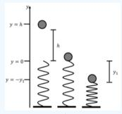
Figure 8.9.1: A ball is dropped from rest onto a vertical spring.
