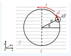
**Figure** 21.9.2 A current-carrying loop in a magnetic field.
