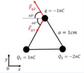
Figure 16.2.3: Force vectors on charge q.
