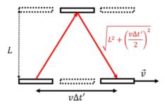
Figure 24.3.2: A clock is made by having a pulse of light bounce back and forth between two parallel mirrors separated by a distance, L. When the clock is placed on a spaceship moving with speed, v, the light travels a longer distance before completing a full cycle, as observed by someone not traveling with the clock.
