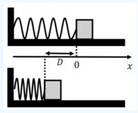
Figure 6.2.8: A block is launched along a frictionless surface by compressing a spring by a distance D. The top panel shows the spring when at rest, and the bottom panel shows the spring compressed by a distance D just before releasing the block.
