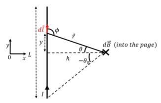
Figure 22.1.2: Setting up the model to use the Biot-Savart Law to calculate the magnetic field a distance h from the center of a current-carrying wire of length L.
