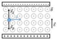
Figure 21.6.2: Illustration of a velocity selector. Only charged particles with a specific speed can make it through without colliding with one of the plates.
