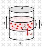
Figure 21.3.1: A section of wire carries conventional current,  $\vec{l}$ , upwards while being immersed in a uniform magnetic field,  $\vec{B}$ , into the page. We introduce the vector,  $\vec{l}$ , to represent a section of wire of length l carrying current in the direction of  $\vec{l}$ .
