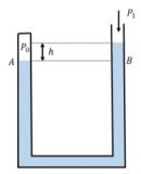
Figure 15.1.10: A barometer constructed from a mamometer to measure relative changes in atmospheric pressure.
