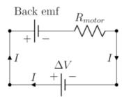
Figure 23.3.1: A simple circuit illustrating how a motor, with resistance,  $R_{motor}$ , will generate a "back emf", equivalent to a battery that produces a voltage in the direction to oppose the current from the actual battery that is powering the motor,  $\Delta V$ .
