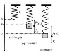
Figure 13.2.1: A vertical spring-mass system.
