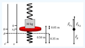
Figure 13.7.3: The forces acting on the platform and our new coordinate system.
