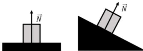
Figure 5.2.2: The normal force, \vec{N} , exerted by a horizontal surface on a block (left side) and by an inclined surface (right side). In both cases, the normal force on the object is perpendicular to the interface between the object and the surface and points in the direction from the interface towards the object.
