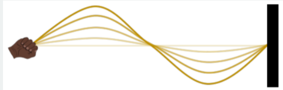
Figure 14.7.2: A standing wave as a stationary wave whose amplitude changes over time.
