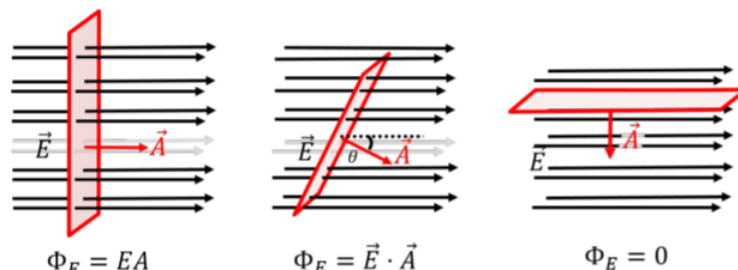
Figure 17.1.1: Flux of an electric field through a surface that makes different angles with respect to the electric field. In the leftmost panel, the surface is oriented such that the flux through it is maximal. In the rightmost panel, there are no field lines crossing the surface, so the flux through the surface is zero.
