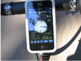
Figure a: / This Global Positioning System (GPS) system, running on a smartphone attached to a bike's handlebar, depends on Einstein's theory of relativity. Time flows at a different rate aboard a GPS satellite than it does on the bike, and the GPS software has to take this into account.
