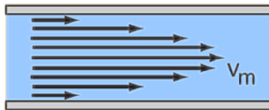
Figure 52.1.1: Laminar fluid flow through a pipe. The maximum flow velocity v_m is at the centerline and is equal to twice the average flow velocity. (Figure from Georgia State University, http://hyperphysics.phy-astr.gsu.edu/hbase/pfric2.html )
