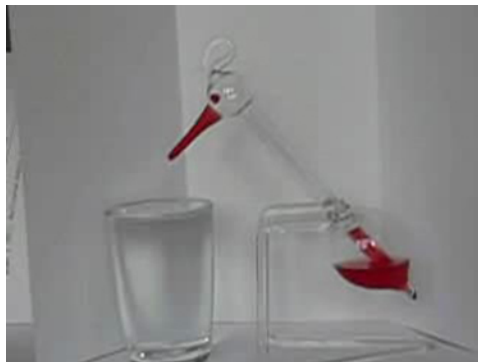
Figure 8.7.11.1: This novelty toy, known as the drinking bird, is an example of Carnot's engine. It contains methylene chloride (mixed with a dye) in the abdomen, which boils at a very low temperature—about 100°F. To operate, one gets the bird's head wet. As the water evaporates, fluid moves up into the head, causing the bird to become top-heavy and dip forward back into the water. This cools down the methylene chloride in the head, and it moves back into the abdomen, causing the bird to become bottom heavy and tip up. Except for a very small input of energy—the original head-wetting—the bird becomes a perpetual motion machine of sorts. (credit: Arabesk.nl, Wikimedia Commons)
