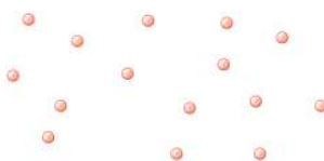
Figure 8.7.3.2: Atoms and molecules in a gas are typically widely separated, as shown. Because the forces between them are quite weak at these distances, the properties of a gas depend more on the number of atoms per unit volume and on temperature than on the type of atom.
