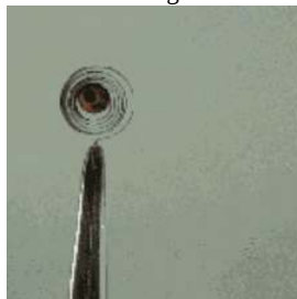
Figure 8.2.6: (a) In an alcohol or mercury thermometer, the liquid (dyed red for visibility) expands when heated and contracts when cooled, much more so than the glass tube that contains the liquid. (b) In a bimetallic thermometer, two different metals (such as brass and steel) form a two-layered strip. When heated or cooled, one of the metals (brass) expands or contracts more than the other metal (steel), causing the strip to coil or uncoil. Both types of thermometers have a calibrated scale that indicates the temperature. (credit a: modification of work by “dwstucke”/Flickr). (c) The demonstration allows one to view the effects of heating and cooling a coiled bimetallic strip. A bimetallic coil from a thermometer reacts to the heat from a lighter, by uncoiling and then coiling back up when the lighter is removed. Animation used with permission from Hustvedt (via Wikipedia).
