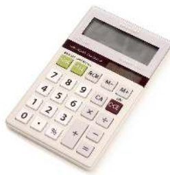
Figure 11.E. 7: The strip of solar cells just above the keys of this calculator convert light to electricity to supply its energy needs. (credit: Evan-Amos, Wikimedia Commons)
