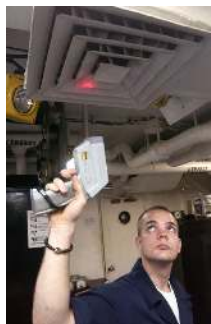
Figure 8.7.2.3: Fireman Jason Ormand uses a pyrometer to check the temperature of an aircraft carrier's ventilation system. Infrared radiation (whose emission varies with temperature) from the vent is measured and a temperature readout is quickly produced. Infrared measurements are also frequently used as a measure of body temperature. These modern thermometers, placed in the ear canal, are more accurate than alcohol thermometers placed under the tongue or in the armpit. (credit: Lamel J. Hinton/U.S. Navy)
