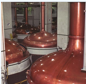
Figure 5.7.3: An oxide of carbon is removed from these fermentation tanks through the large copper pipes at the top. (credit: "Dual Freq"/Wikimedia Commons)
