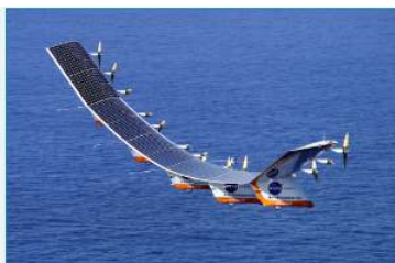
Figure 8.4.2.2 Solar energy is converted into electrical energy by solar cells, which is used to run a motor in this solar-power aircraft. (credit: NASA)
