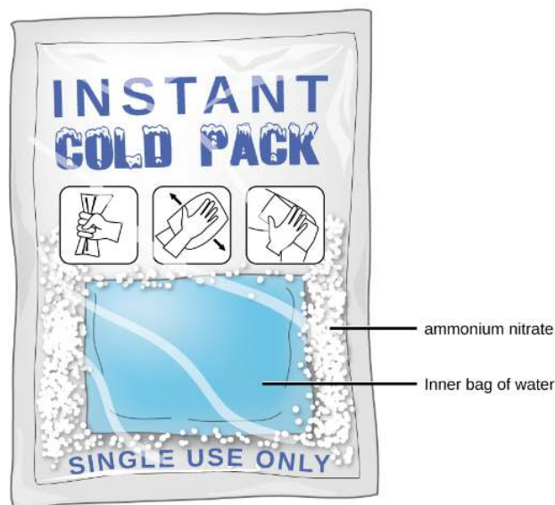
Figure 7.2.5: An instant cold pack gets cold when certain salts, such as ammonium nitrate, dissolve in water—an endothermic process. This figure shows a single use instant cold pack with labels indicating an inner bag of water surrounded by white particulate ammonium nitrate.
