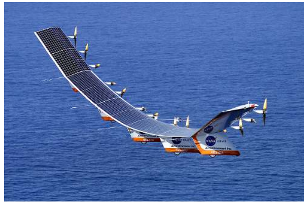
Figure 8.8.1: Solar energy is converted into electrical energy by solar cells, which is used to run a motor in this solar-power aircraft. (credit: NASA)
