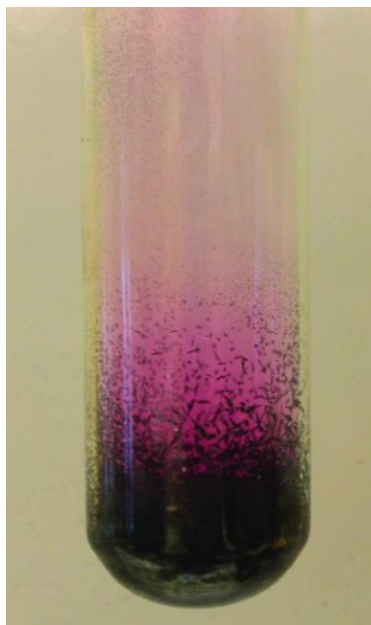
Figure 4.7.6: Sublimation of solid iodine in the bottom of the tube produces a purple gas that subsequently deposits as solid iodine on the colder part of the tube above. (credit: modification of work by Mark Ott)
