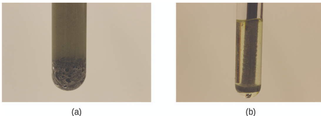
Figure 6.8.1: (a) Iron powder reacts rapidly with dilute hydrochloric acid and produces bubbles of hydrogen gas: 2\text{Fe(s)} + 6\text{HCl(aq)} \rightarrow 2\text{FeCl}_3\text{(aq)} + 3\text{H}_2\text{(g)} . (b) An iron nail reacts more slowly because the surface area exposed to the acid is much less.
