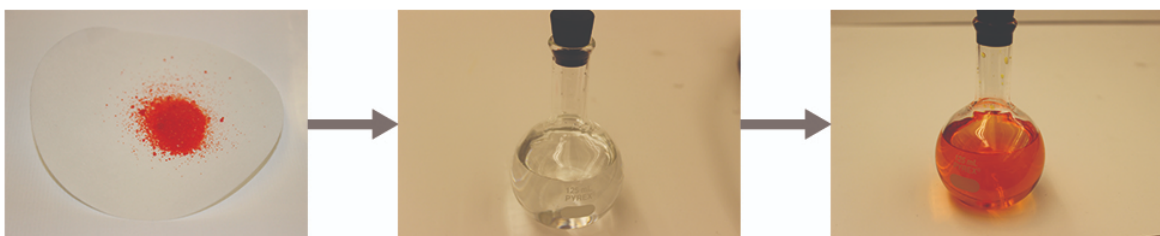
Figure 7.2.1: When potassium dichromate ( K_2Cr_2O_7 ) is mixed with water, it forms a homogeneous orange solution. (credit: modification of work by Mark Ott). The first photo shows a small mound of an orange crystalline solid. There is a right-facing arrow. The second photo shows a translucent, colorless liquid in a clear container. There is a right-facing arrow. The third photo shows a translucent orange liquid in a clear, covered container.
