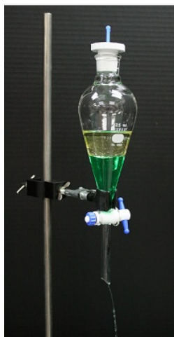
Figure 5.2.1: Separatory Funnel containing oil and colored water to display density differences. (CC BY-SA 3.0; PRHaney via Wikipedia ).
