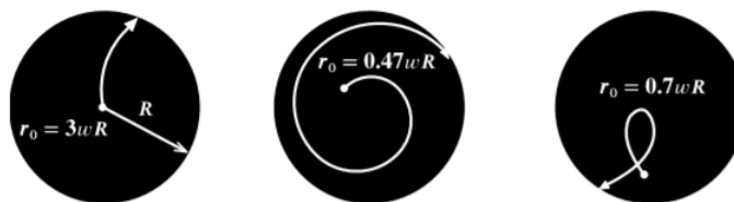
Figure 12.8.1: Free-force motion of a hockey puck sliding on a rotating frictionless table of radius R that is rotating with constant angular frequency \omega out of the page.
