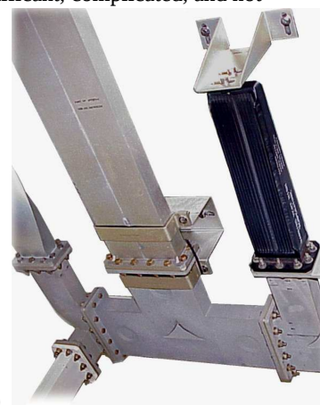
Figure 21.4.5 A network of radio frequency waveguides in an air traffic control radar. (CC BY SA 2.0 Germany)
