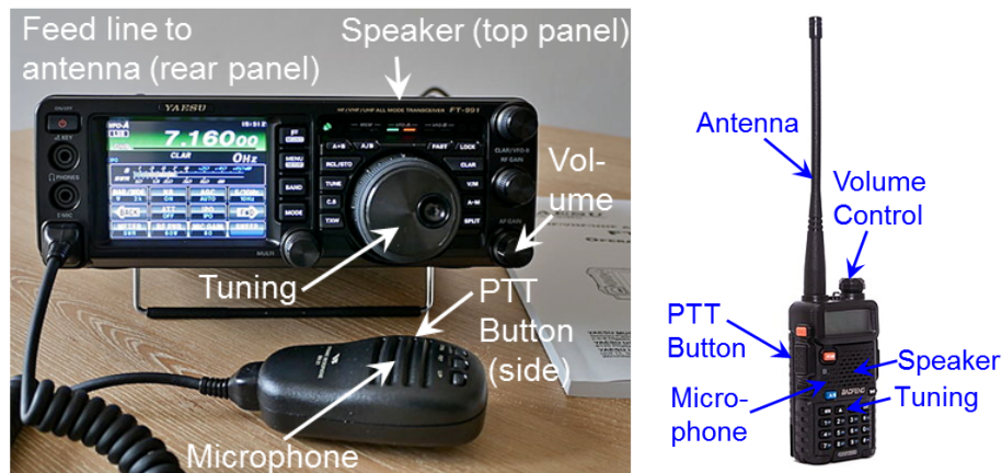
Figure 1.5.2: (left to right) Examples of an Amateur Radio base-station transceiver [2] and handheld transceiver [3]. For the base-station transceiver, the feed line connects to the back of the unit and is not shown. For the handheld transceiver, the feed line is just the connector from the antenna to the unit.
