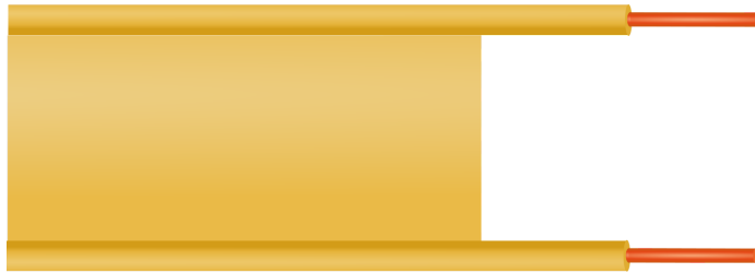
Figure 21.15.1 Twin lead, a commonly-encountered form of parallel wire transmission line. (CC BY SA 3.0 (modified); SpinningSpark)
