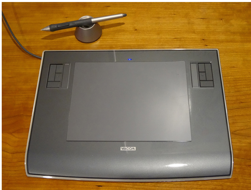
Figure 9.10.1: A tablet with a specially designed pen to write with is another application of magnetic induction.
