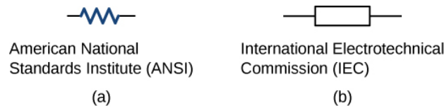
Figure 5.4.2: Symbols for a resistor used in circuit diagrams. (a) The ANSI symbol; (b) the IEC symbol.
