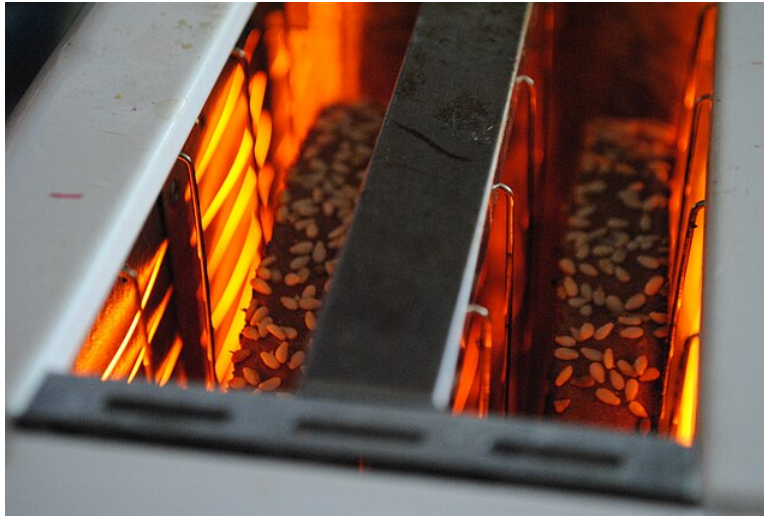
Figure 5.1.1: Current flowing through resistive elements in a toaster cause them to give off heat and light. [1]
