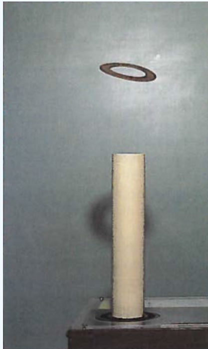
Figure 9.4.4: The jumping ring. When a current is turned on in the vertical solenoid, a current is induced in the metal ring. The stray field produced by the solenoid causes the ring to jump off the solenoid.
