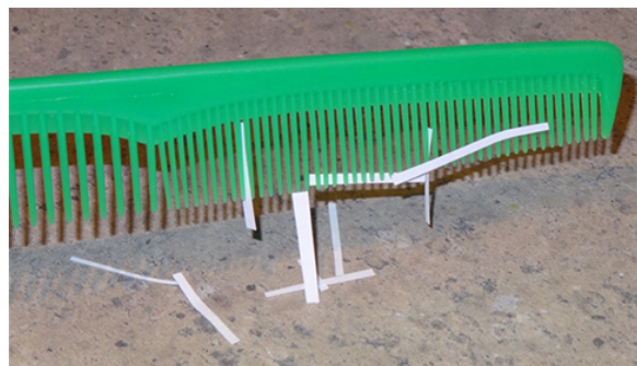
Figure 2.2.2: After being used to comb hair, this comb attracts small strips of paper from a distance, without physical contact. Investigation of this behavior helped lead to the concept of the electric force.
