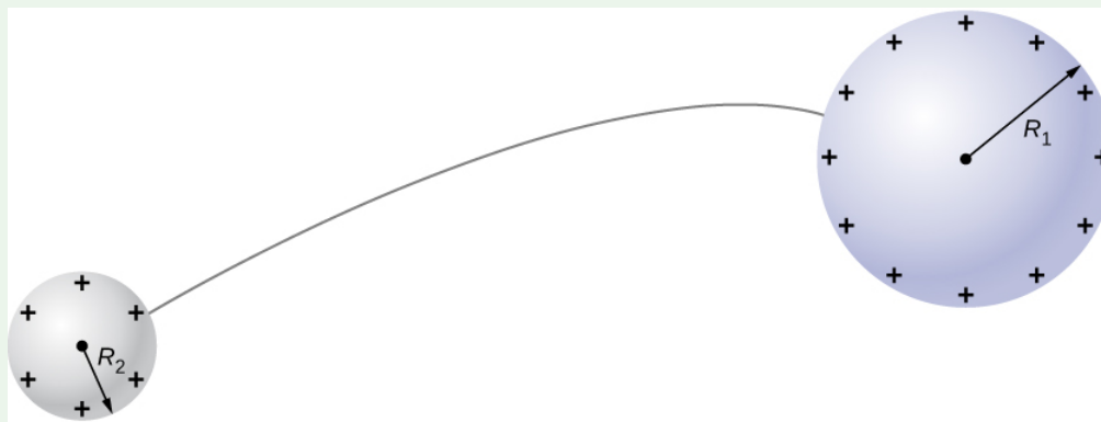
Figure 4.4.5: Two conducting spheres are connected by a thin conducting wire.
