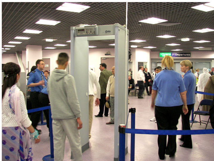
Figure 10.3.5: The familiar security gate at an airport not only detects metals, but can also indicate their approximate height above the floor. (credit: “Alexbuidrs”/Wikimedia Commons)
