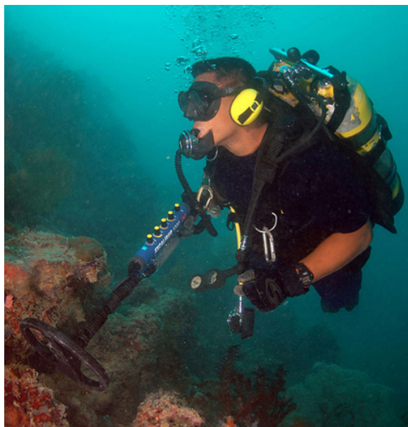
Figure [Math Processing Error]: When a metal detector comes near a piece of metal, the self-inductance of one of its coils changes. This causes a shift in the resonant frequency of a circuit containing the coil. That shift is detected by the circuitry and transmitted to the diver by means of the headphones.
