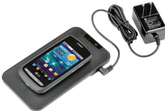
Figure 10.1.1: A smartphone charging mat contains a coil that receives alternating current, or current that is constantly increasing and decreasing. The varying current induces a source voltage in the smartphone, which charges its battery. Note that the black box containing the electrical plug also contains a transformer that modifies the current from the outlet to suit the needs of the smartphone. (credit: modification of work by “LG”/Flickr)
