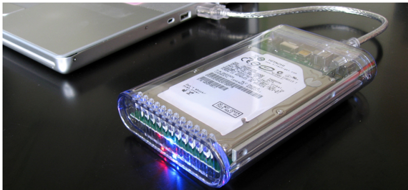
Figure 18.1.1: An external hard drive attached to a computer works by magnetically encoding information that can be stored or retrieved quickly. A key idea in the development of digital devices is the ability to produce and use magnetic fields in this way. (credit: modification of work by “Miss Karen”/Flickr)
