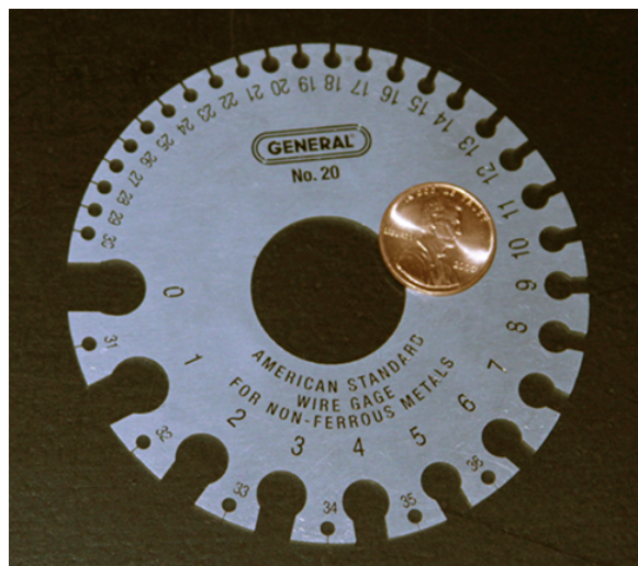
Figure 5.3.5: A device for measuring the gauge of electrical wire. As you can see, higher gauge numbers indicate thinner wires.
