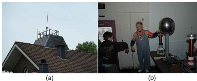
Figure 4.5.4: (a) A lightning rod is pointed to facilitate the transfer of charge. (credit: Romaine, Wikimedia Commons) (b) This Van de Graaff generator has a smooth surface with a large radius of curvature to prevent the transfer of charge and allow a large voltage to be generated. The mutual repulsion of like charges is evident in the person's hair while touching the metal sphere. (credit: Jon 'ShakataGaNaI' Davis/Wikimedia Commons).
