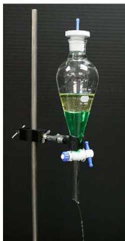
Figure 20.2.1: Separatory Funnel containing oil and colored water to display density differences. (CC BY-SA 3.0; PRHaney via Wikipedia ).
