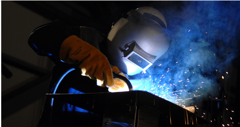
Figure 14.1.1: The welder's gloves and helmet protect him from the electric arc that transfers enough thermal energy to melt the rod, spray sparks, and burn the retina of an unprotected eye. The thermal energy can be felt on exposed skin a few meters away, and its light can be seen for kilometers. (credit: Kevin S. O'Brien/U.S. Navy)
