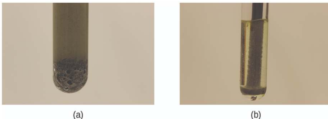
Figure 21.8.1: (a) Iron powder reacts rapidly with dilute hydrochloric acid and produces bubbles of hydrogen gas: 2\text{Fe(s)} + 6\text{HCl(aq)} \rightarrow 2\text{FeCl}_3\text{(aq)} + 3\text{H}_2\text{(g)} . (b) An iron nail reacts more slowly because the surface area exposed to the acid is much less.
