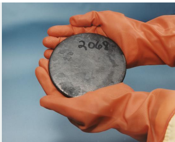
Figure 15.7.3: A billet of highly enriched uranium that was recovered from scrap processed at the Y-12 National Security Complex Plant. Original and unrotated.
