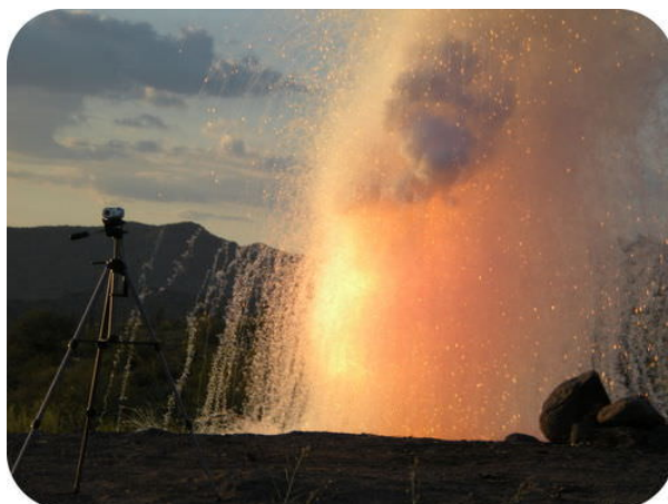
Figure 10.6.2: Pictured here is about 3 pounds of sodium metal reacting with water. Sodium metal reacts vigorously when dropped into a container of water, giving off hydrogen gas. A large piece of sodium will often generate so much heat that the hydrogen will
