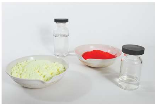
Figure 20.3.5 Each sample contains 6.022 \times 10^{23} molecules or formula units—1.00 mol of the compound or element. Clock-wise from the upper left: 130.2 g of \text{C}_8\text{H}_{17}\text{OH} (1-octanol, formula mass 130.2 amu), 454.4 g of \text{HgI}_2 (mercury(II) iodide, formula mass 454.4 amu), 32.0 g of \text{CH}_3\text{OH} (methanol, formula mass 32.0 amu) and 256.5 g of \text{S}_8 (sulfur, formula mass 256.5 amu). (credit: Sahar Atwa).
