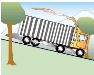
Figure 14.6.2: The smoking brakes on this truck are a visible evidence of the mechanical equivalent of heat.
