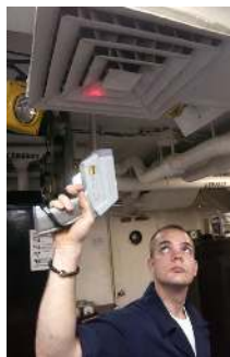
Figure 14.2.3: Fireman Jason Ormand uses a pyrometer to check the temperature of an aircraft carrier's ventilation system. Infrared radiation (whose emission varies with temperature) from the vent is measured and a temperature readout is quickly produced. Infrared measurements are also frequently used as a measure of body temperature. These modern thermometers, placed in the ear canal, are more accurate than alcohol thermometers placed under the tongue or in the armpit. (credit: Lamel J. Hinton/U.S. Navy)
