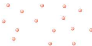
Figure 14.3.2: Atoms and molecules in a gas are typically widely separated, as shown. Because the forces between them are quite weak at these distances, the properties of a gas depend more on the number of atoms per unit volume and on temperature than on the type of atom.
