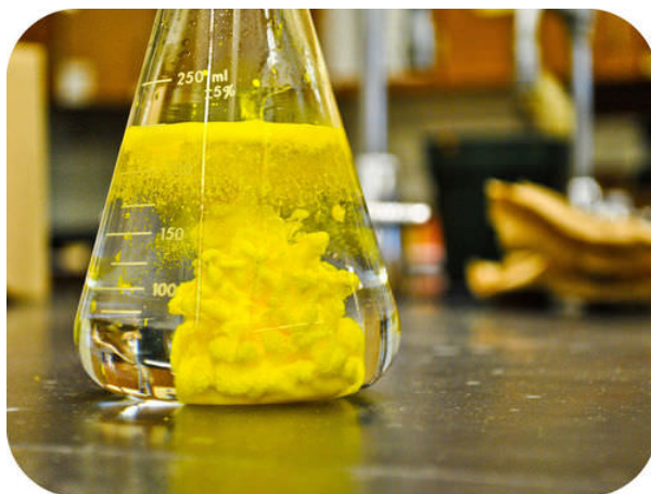
Figure 10.6.3: When a few drops of lead (II) nitrate are added to a solution of potassium iodide, a yellow precipitate of lead (II) iodide immediately forms in a double-replacement reaction.
