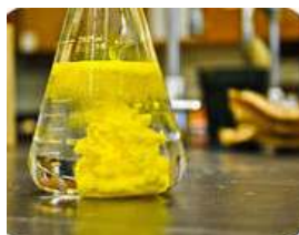
Figure 10.4.6: A yellow precipitate of solid lead (II) iodide forms immediately when solutions of lead (II) nitrate and potassium iodide are mixed.
