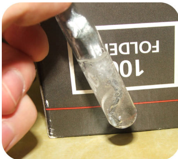
Figure 10.6.1: Zinc metal reacts with hydrochloric acid to give off hydrogen gas in a single-replacement reaction.
