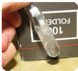
Figure 10.4.5: Zinc reacts with hydrochloric acid to produce bubbles of hydrogen gas.
