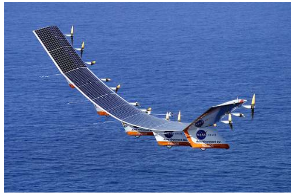
Figure 5.6.1: Solar energy is converted into electrical energy by solar cells, which is used to run a motor in this solar-power aircraft. (credit: NASA)
