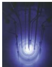
Figure 10.9.7: The blue glow in this research reactor pool is Cerenkov radiation caused by subatomic particles traveling faster than the speed of light in water. (credit: U.S. Nuclear Regulatory Commission)
