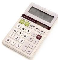
Figure 7.E. 7: The strip of solar cells just above the keys of this calculator convert light to electricity to supply its energy needs. (credit: Evan-Amos, Wikimedia Commons)
