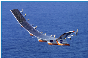
Figure 5.3.2: Solar energy is converted into electrical energy by solar cells, which is used to run a motor in this solar-power aircraft. (credit: NASA)
