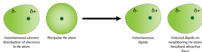
Figure 19.9.3 A short-lived or instantaneous dipole in a helium atom. (CC
