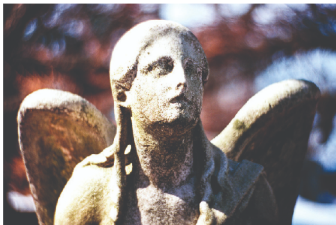
Figure 21.8.2 Statues made from carbonate compounds such as limestone and marble typically weather slowly over time due to the actions of water, and thermal expansion and contraction. However, pollutants like sulfur dioxide can accelerate weathering. As the concentration of air pollutants increases, deterioration of limestone occurs more rapidly. (credit: James P Fisher III)
