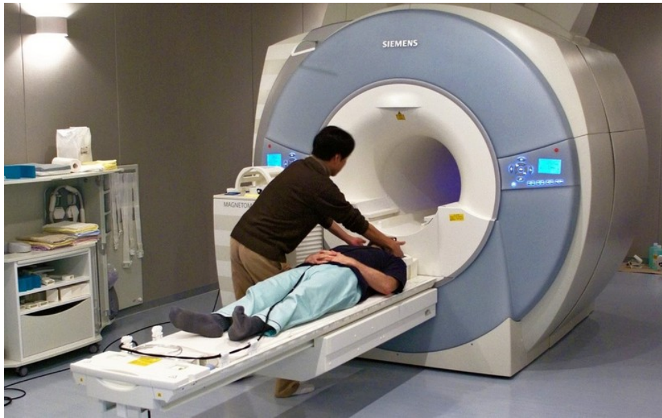
Figure 12.9.3: Functional magnetic resonance imaging (fMRI) scanner used to image the brain while people perform tasks. The scanner allows researchers to view the changes in blood oxygenation in specific locations in the brain during a task. Images are collected using powerful magnets and radio waves that shift the position of atoms in oxygenated blood that rushes to areas involved in performing the task. MRIs are non-invasive and there are no known risks from exposure to the magnetic fields or radio waves. Subjects lay on the while bed with their head inside the head coil, then the bed is moved into the scanner. [Image: Janne Moren, https://goo.gl/MKb2jn , CC BY-NC-SA 2.0, goo.gl/Toc0ZF ]
