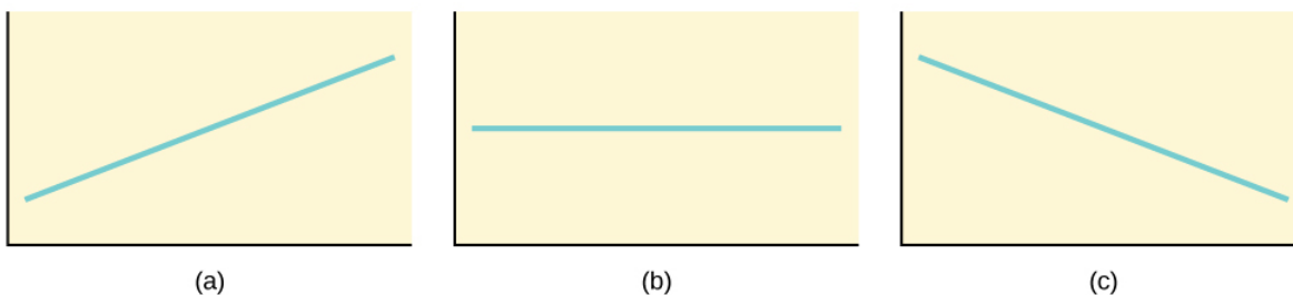
Figure 12.1.3: Three possible graphs of y = a + bx (a) If b > 0 , the line slopes upward to the right. (b) If b = 0 , the line is horizontal. (c) If b < 0 , the line slopes downward to the right.
