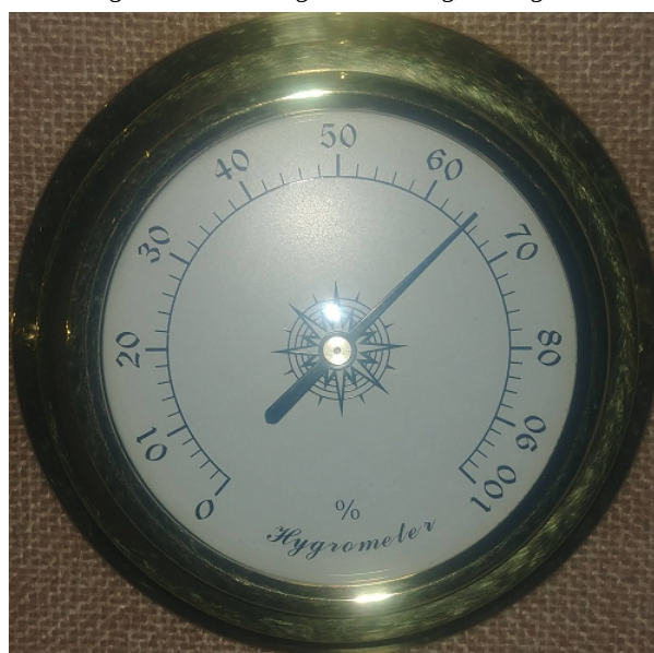
Figure 3.1.4: Hygrometer showing office humidity at 65 percent, example of ratio data type.
