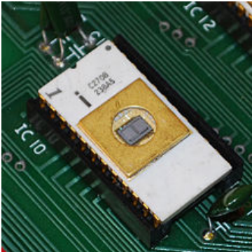
An Intel 2708 EPROM “chip” on a circuit board.
