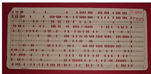
Initial program load punched card for the IBM 1130 (1965)
