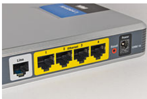
A typical home or small office router showing the ADSL telephone line and Ethernet network
