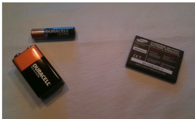
Figure 2: Primary versus Secondary Batteries. Primary batteries (left) are non-rechargeable and disposable. Secondary batteries (right) are rechargeable, like this cellular phone battery.
